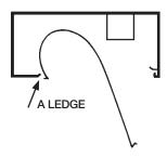
**10.** Squeeze reflector back into housing.
