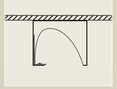
Ideal placement is 8" to 12" from the front edge of fixture to the surface you are lighting, at 8' to 10' height.
