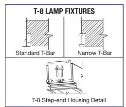
RECESSED Display Wall Wash/Grazer for T-Bar Lay-in Fluorescent Fixtures
