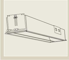
Ideal placement is 8" to 12" from the front edge of fixture to the surface you are lighting, at 8' to 10' height.
