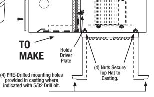
2. Casting has PRE-Drill Mounting Holes to secure to studs with drywall screws (by others). Remove lid of "Top Hat" to secure it to the Casting with provided nuts. This can be done before or after securing the Casting to the studs depending on your plenum height to be able to secure the Top Hat. Then secure the lid.
