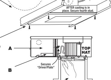
Remove Lens/Frame <u>FIRST</u> if you must access the LED or Driver Plate. Remove the lens by <u>pushing</u> it up slightly to grab edge of lens frame and pull down to dislodge from clips and carefully pull down.
