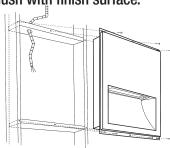
**3.** Finish the building exterior and paint fixture to match (lower light levels occur with dark paint).
