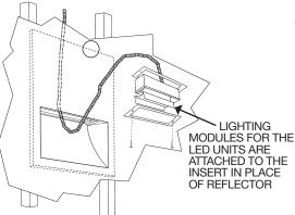
**5.** To apply a finish to the face of fixture to match the exterior building, use "Weld-Crete" and follow the manufacturer's instructions.
