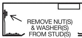
4. This will allow you to tilt the LED Bracket forward and remove. To replace the driver a “quick connect” to disconnect power is provided.
