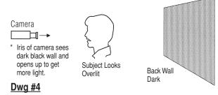
**Solutions** – To accomplish the above requires light fixtures that provide a wide horizontal component. The VT Series fixture ENGINEERED LIGHTING PRODUCTS has designed for this use is a recessed, indirect  $2^{'}$  x  $2^{'}$  with a 44 watt LED or two 40, 50
