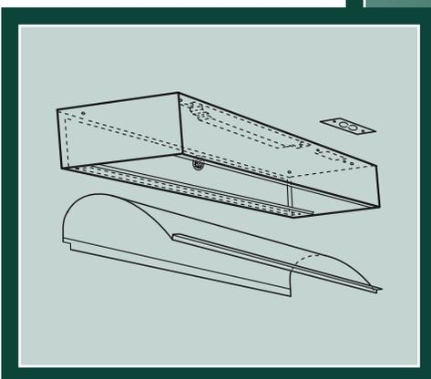
*Ideal placement is 24" to 36" from the front edge of fixture to the surface you are lighting, for 8' to 12' ceilings.*
